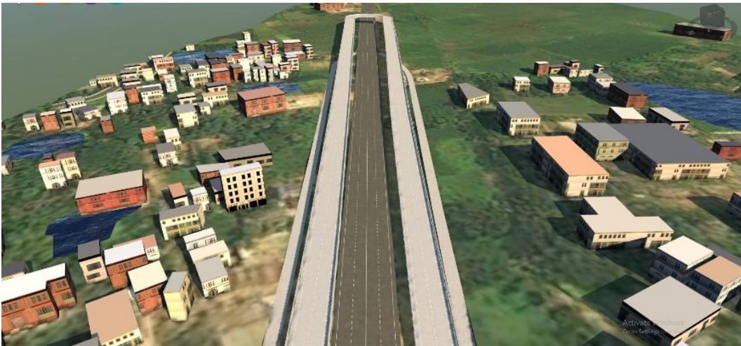
Figure 4. Grade separated U-loop facility.
