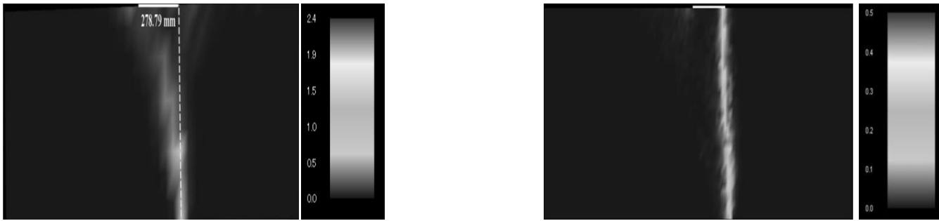
(a) (b) Figure 10. Development of shear band at 60 mm (a) without structure (b) with structure.
