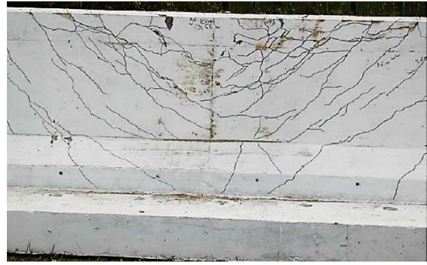
(a) (b) Figure 1. (a) Pendulum impact test on barrier, and (b) cracks pattern of the tested GFRP reinforced barrier (El-Salakawy et al. 2001)
