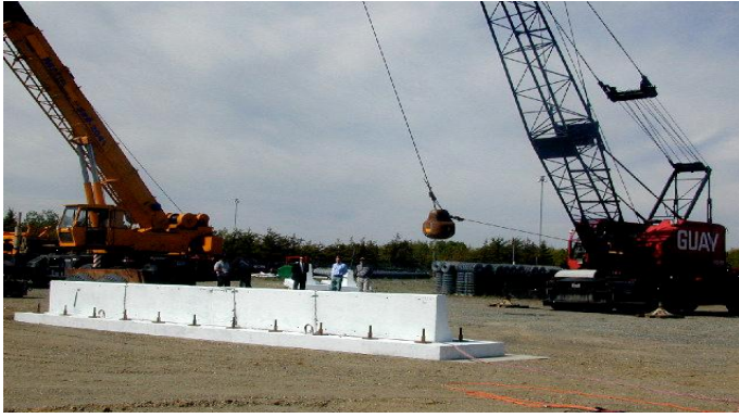
(a) (b) Figure 1. (a) Pendulum impact test on barrier, and (b) cracks pattern of the tested GFRP reinforced barrier (El-Salakawy et al. 2001)
