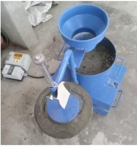
Figure 1. Measuring vebe time of RCC.
