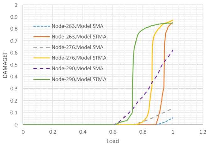
Figure 11. Damage progression rate in girder.
