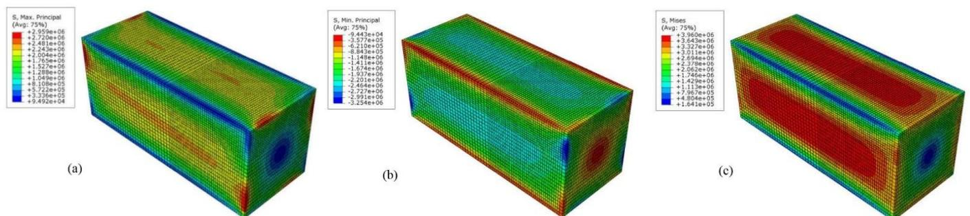
Figure 6.(a) Maximum principal stress. (b) Minimum principal stress. (c) Von Mises Stress, of *Model T*.
