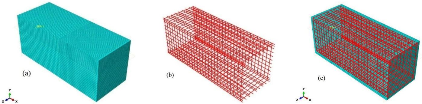
Figure 5. FE model of (a) concrete girder (b) reinforcement (c) assembled girder and reinforcement.
