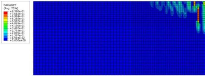
Figure 9. Crack patterns of girder for *Model SMA* (Side Elevation)
