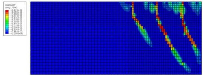
Figure 10. Crack patterns of girder for *Model STMA* (Side Elevation)
