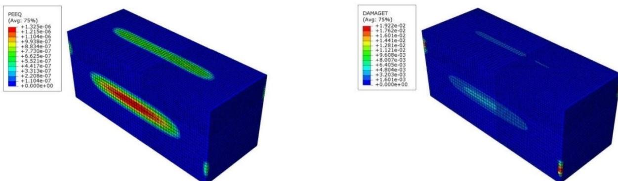
Figure 7. Equivalent plastic strain for *Model T*.
