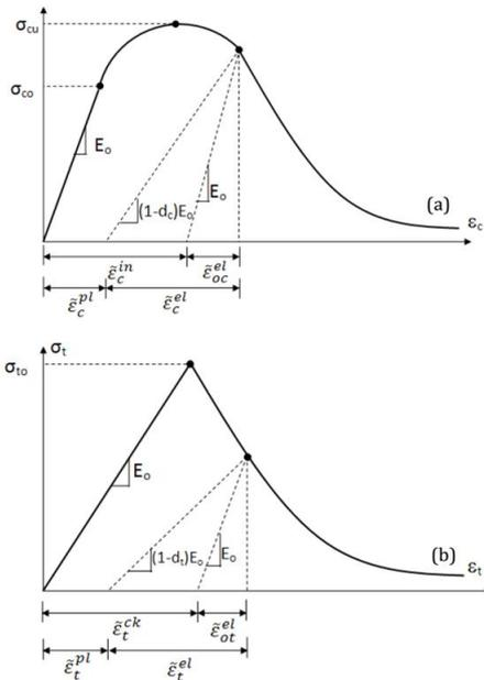
Figure 3. (a) Uniaxial compressive and (b) Uniaxial tensile performance of concrete.
