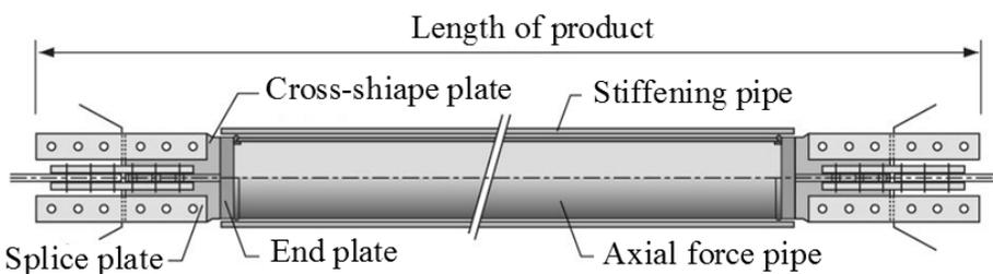
Figure 4. Structure of buckling restraint bracing.
