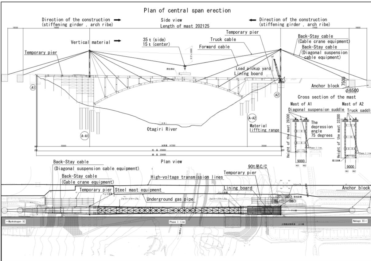
Figure 13. Plan of central span erection.
