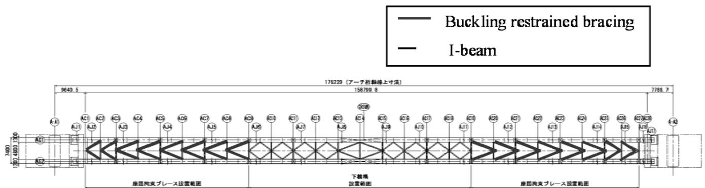
Figure 6. The location where I located buckling restraint bracing.
