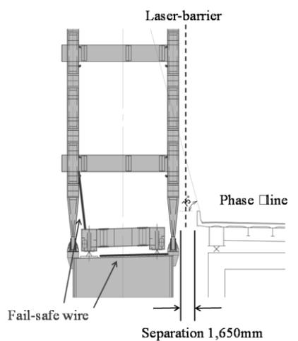
Figure 15. Fail-safe of the mast.
