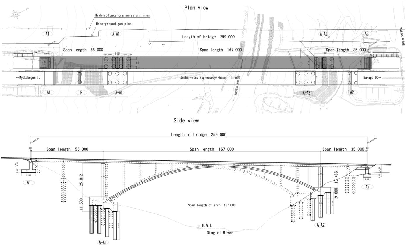
Figure 1. Figure of bridge public (plan view and side view).
