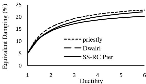
Figure 9. Comparison of damping-ductility curve.
