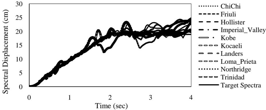
Figure 7. Displacement spectra of ten earthquake records matched with target response spectrum.
