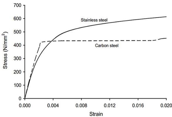
Figure 1. Typical mechanical properties of carbon steel and stainless steel.
