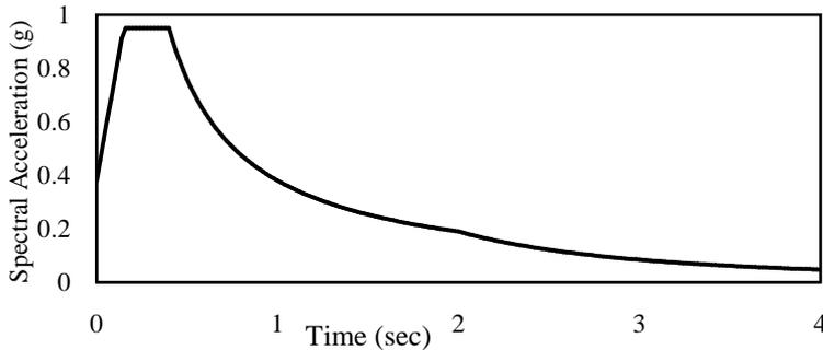
Figure 5. Design acceleration response spectrum.
