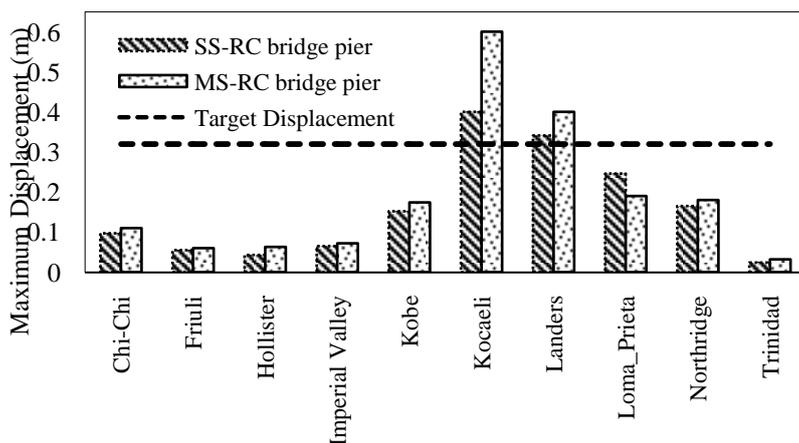
Figure 11. Maximum structural displacement for SS RC bridge pier compared with MS-RC bridge pier.
