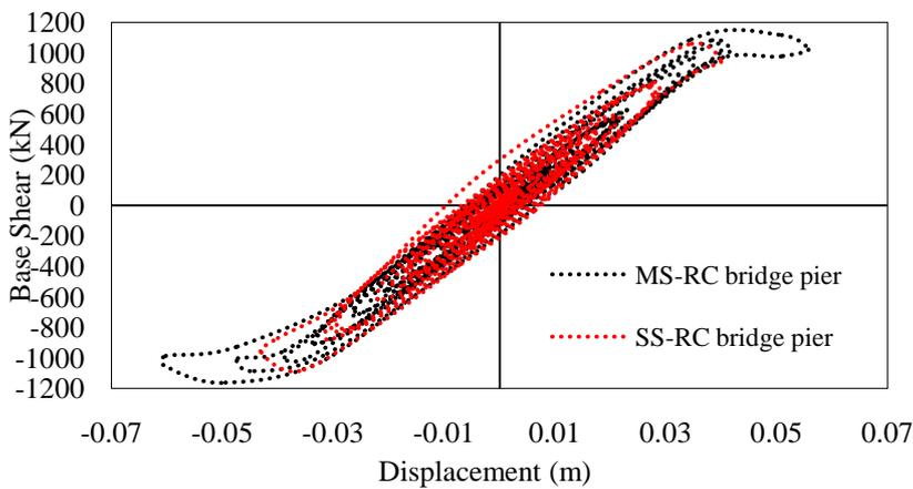
Figure 10. Hysteretic behavior of SS-RC bridge pier and MS RC bridge pier.
