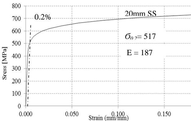
Figure 3. Mechanical properties of stainless steel grade 201.
