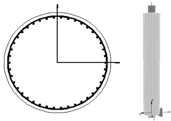
Figure 4. Cross section and elevation of SS reinforced concrete bridge pier.
