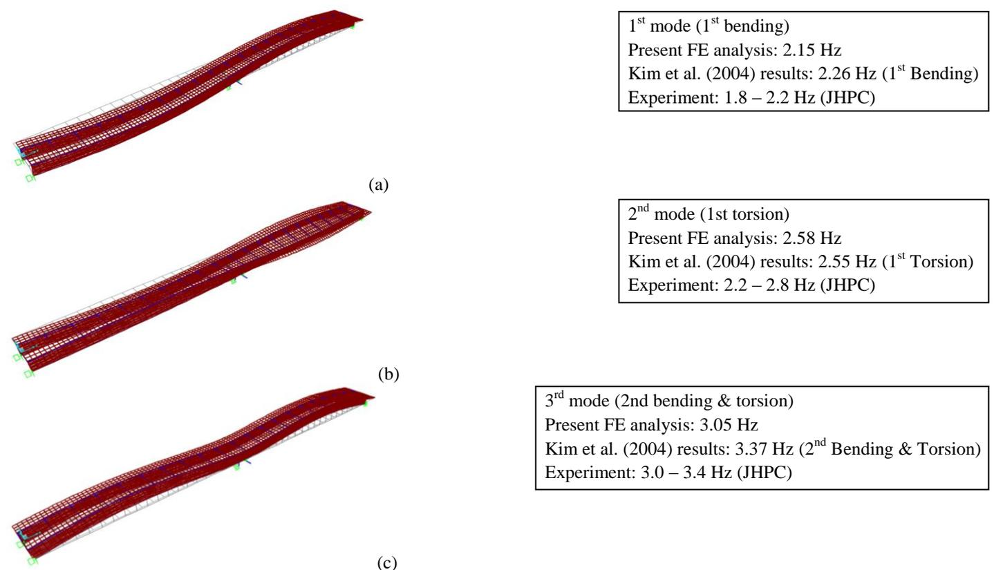
Figure 2. Comparison of present natural vibration frequencies and mode shapes with past FEM and experimental results.
