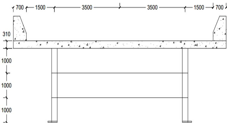
Figure 1. Cross-section of the bridge deck (mm).
