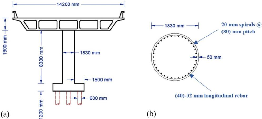
Figure 1. Bridge pier: (a) elevation and (b) cross section.
