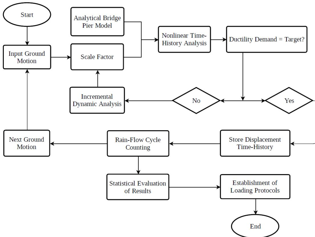
Figure 3. Flow chart of methodology for the development of loading protocols.
