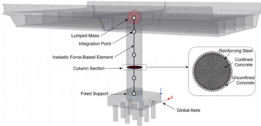
Figure 2. Analytical model scheme of the bridge pier.
