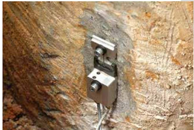
Fig 11. Final setup of combined acceleration and strain sensor
