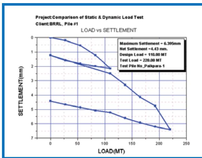
Fig 7. SLT of Pile#1
