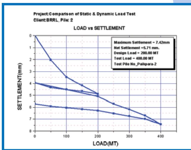
Fig 7. SLT of Pile#1
