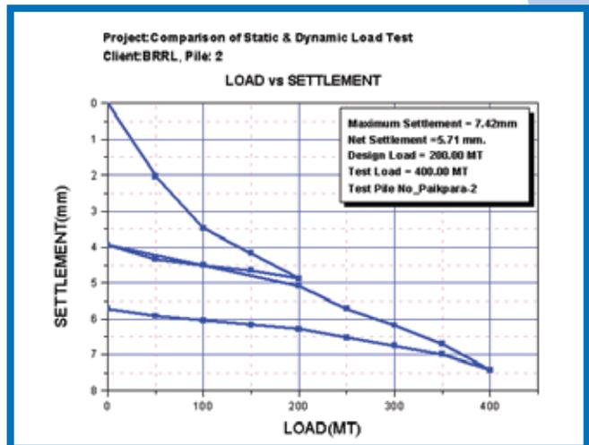
Fig 7. SLT of Pile#2
