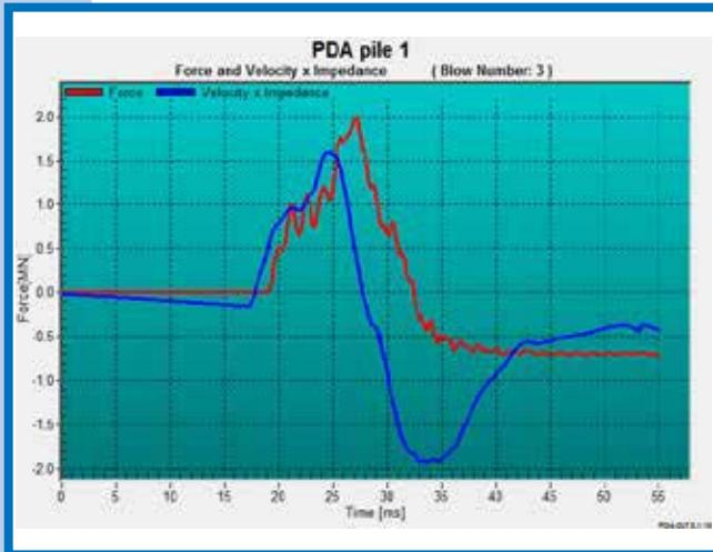
Fig 13. Load vs. Time of Pile#1
