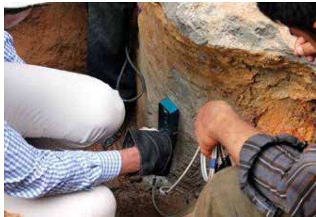
Fig 10. Preparation of combined acceleration and strain sensor
