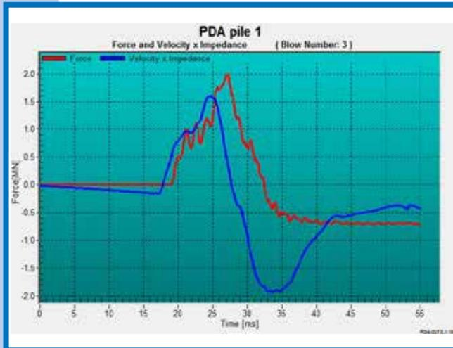
Fig 13. Load vs. Time of Pile#1
