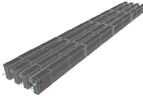
Figure 6. FE model of 2<sup>nd</sup> span.
