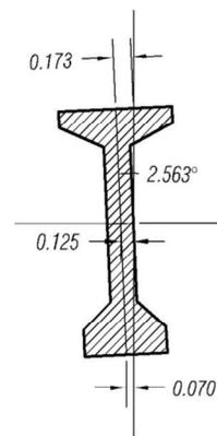
Figure 2a. Section at first quarter span.
