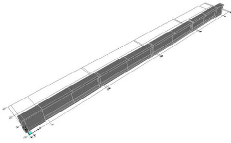
Figure 5. FE model of single girder
