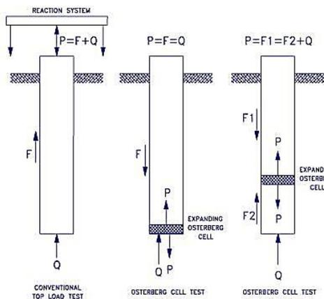
Figure 2. Conventional and O-cell test.
