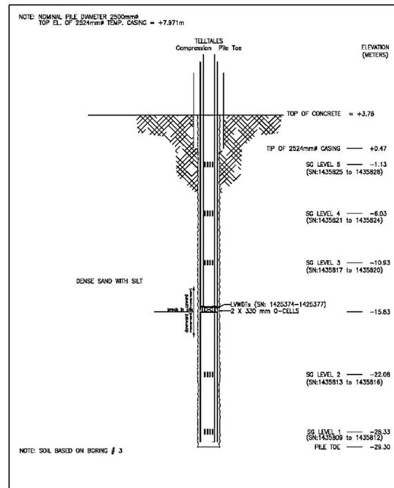
Figure 3. Load Transfer Zone and of strain gauge
