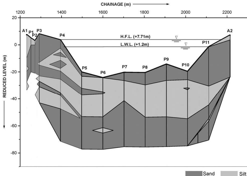
Figure 1. Generalized cross sectional profile at boring locations.
