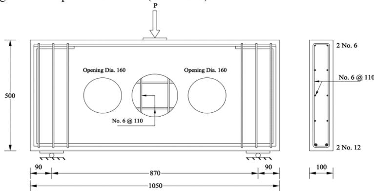
Figure 2. Group B beam details (unit in mm)
