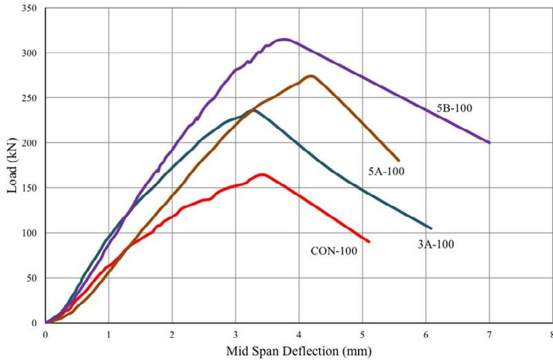
Figure 9. Load deflection response of Group A beams
