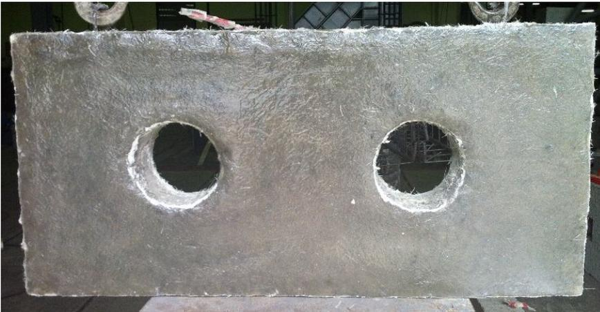
Figure 4. Typical SFRP strengthened RC deep beam with openings
