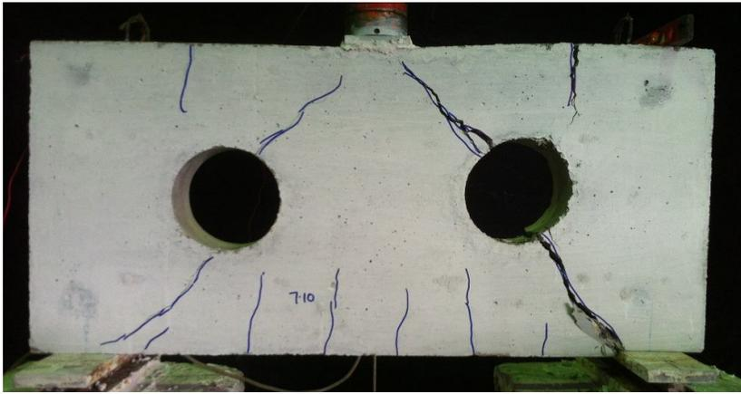
Figure 13. Un-strengthened beam specimen (openings size = 160 mm diameter)
