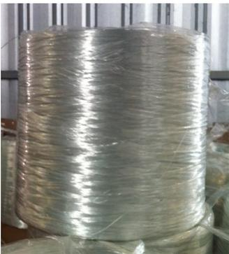
Figure 5. Glass fiber roving
