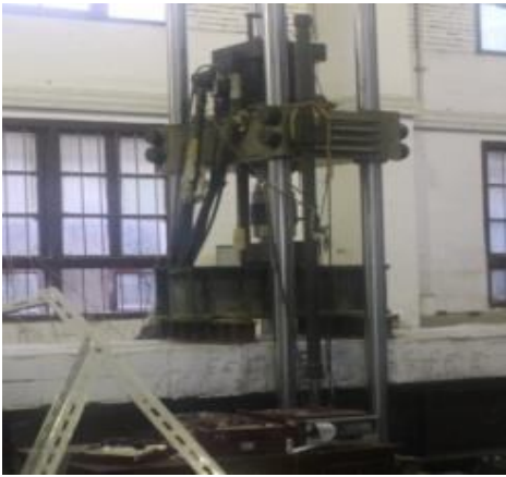
Figure 4. Load device of fatigue experiment
