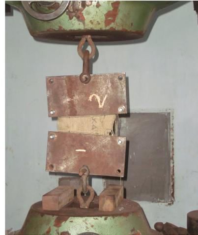
Figure 15. Experimental setup of tension test of JUTE sheet
