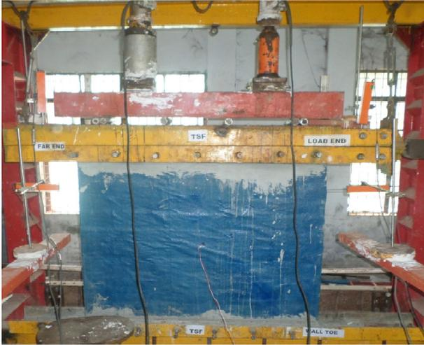
Figure 14. Experimental setup of COTTON-FRP reinforced shear wall
