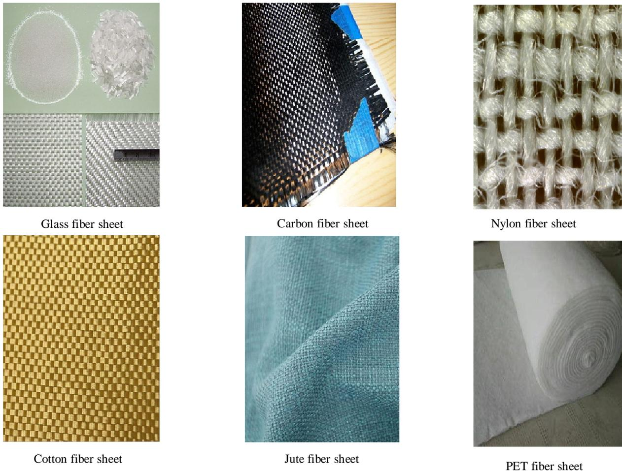
Figure 4. Common types of fiber sheet
