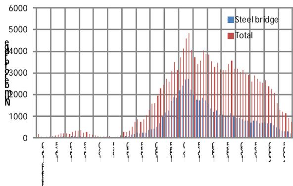
Figure 1. The number of highway bridges by construction year (NILIM,2015)
