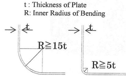
Figure 4. Minimum radius of cold bending
