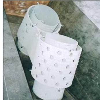
Figure 6. Double steel-pipe joint system
