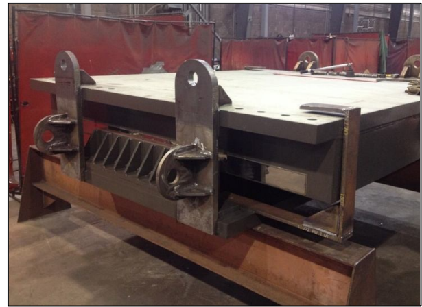
Figure 10. Wind restrained installed in bearing
