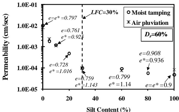
Figure 4. Permeability test results of sand and silt mixtures
