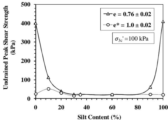
Figure 7. Peak deviator stress verses silt content at constant  $e$  and  $e^*$ .
