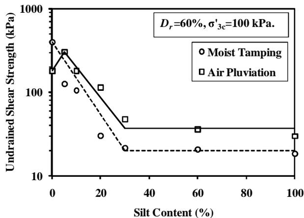
Figure 3. Peak shear stress verses silt content for specimens prepared by moist tamping and air pluviation methods
