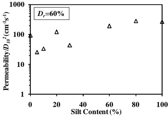
Figure 6. Normalized coefficient of permeability vs. Silt content
