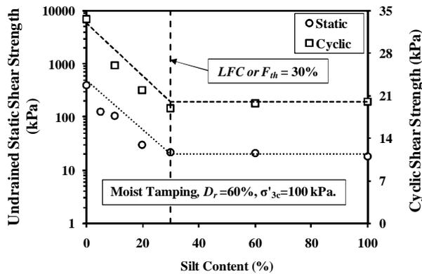
Figure 2. (a) Cyclic and (b) static triaxial test results
