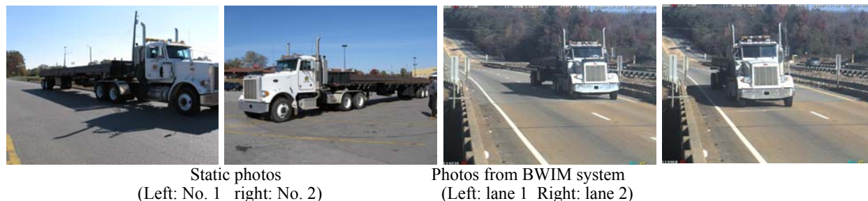
Figure 4. Vehicles for the initial calibration of bridge on highway I-78
