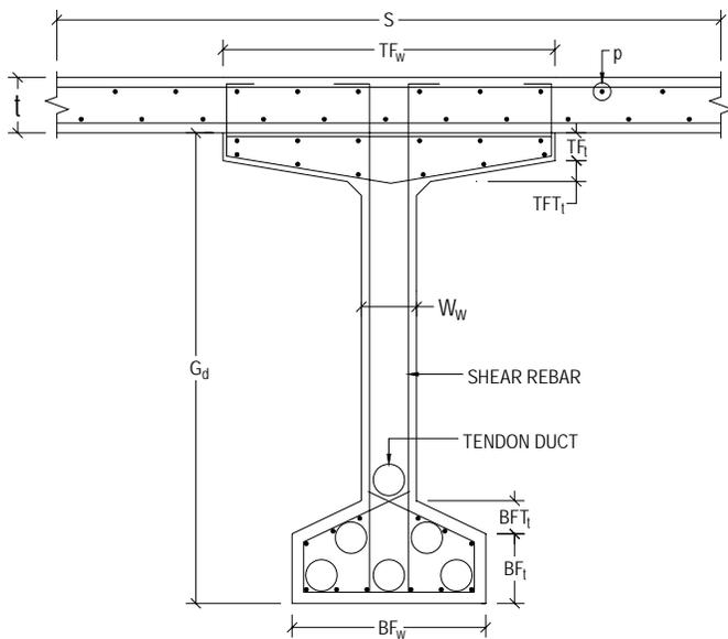
Figure 4. Girder composite section with design variables.
