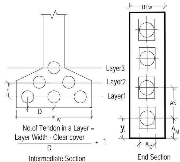
Figure 5. Tendons arrangement in the girder
