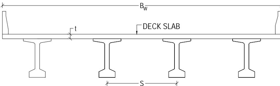
Figure 6. Girders arrangement in the bridge
