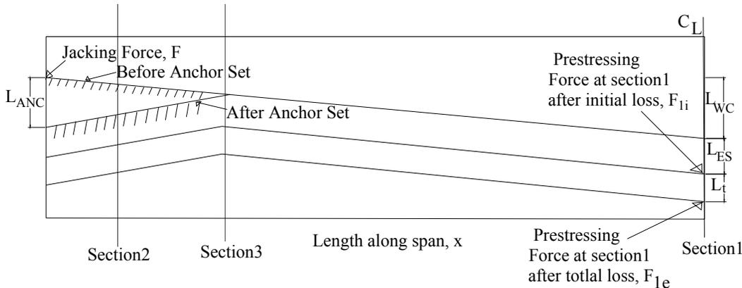
Figure 8. Variation of prestressing force along the length of girder
