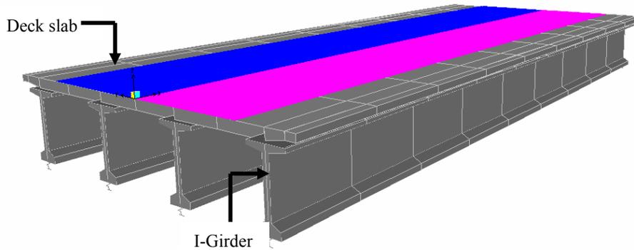
Figure 2. Prestressed concrete I-Girder bridge system.
