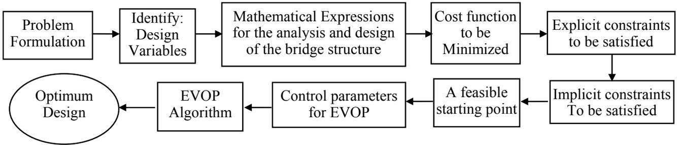
Figure 3. Optimization Problem Formulation and Linking with EVOP
