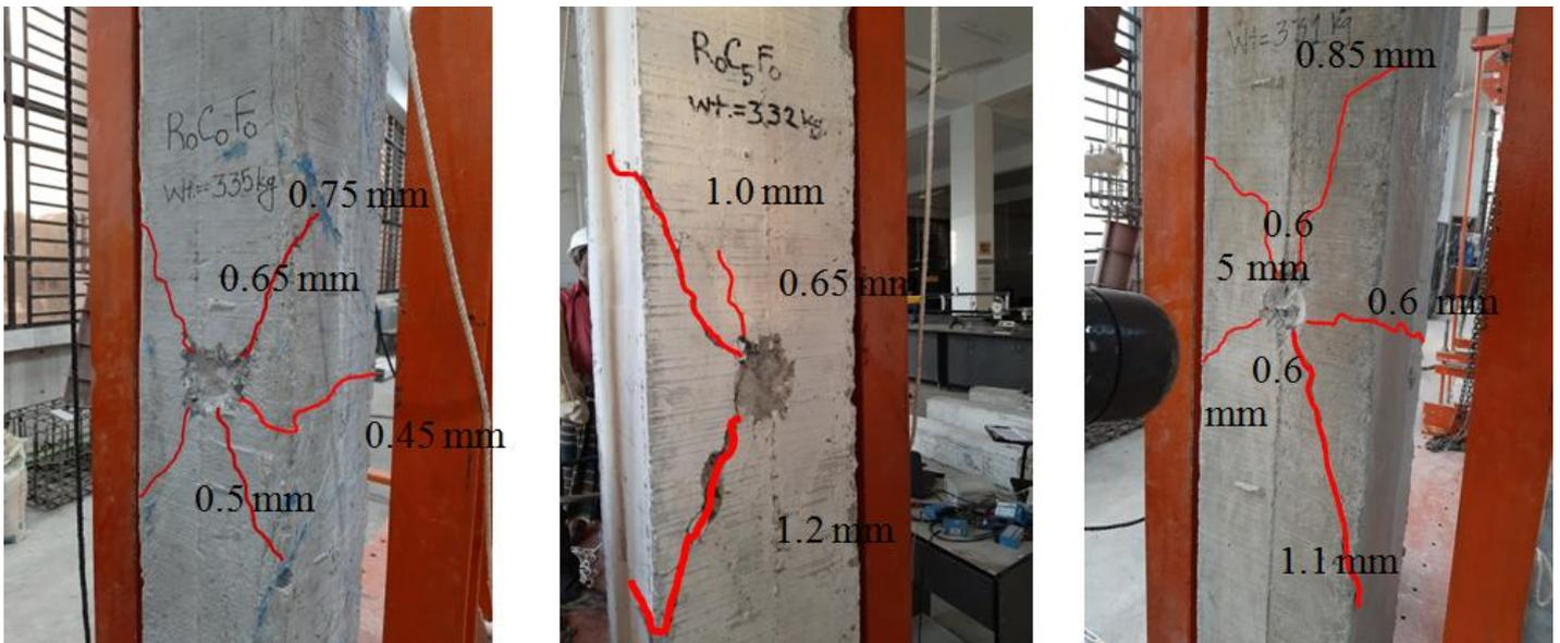
Figure 6. Failure pattern of test specimens (a) Control (b) Specimens with only CR (c) Specimens with combination of RCA, CR and PPF.
