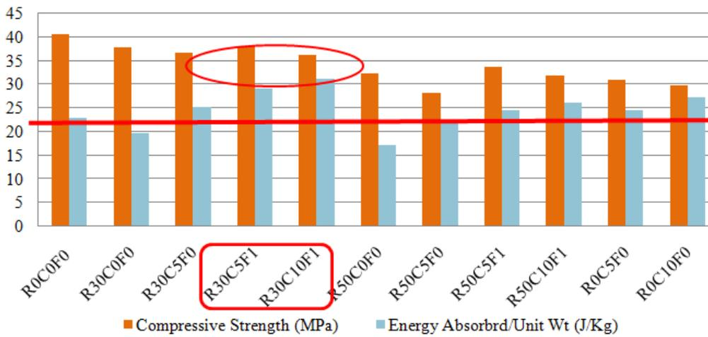
Figure 2. Comparison of compressive strength and energy absorption capacity.
