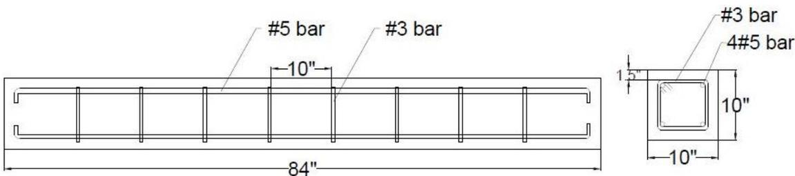
Figure 1. Reinforcement detailing of test specimens.
