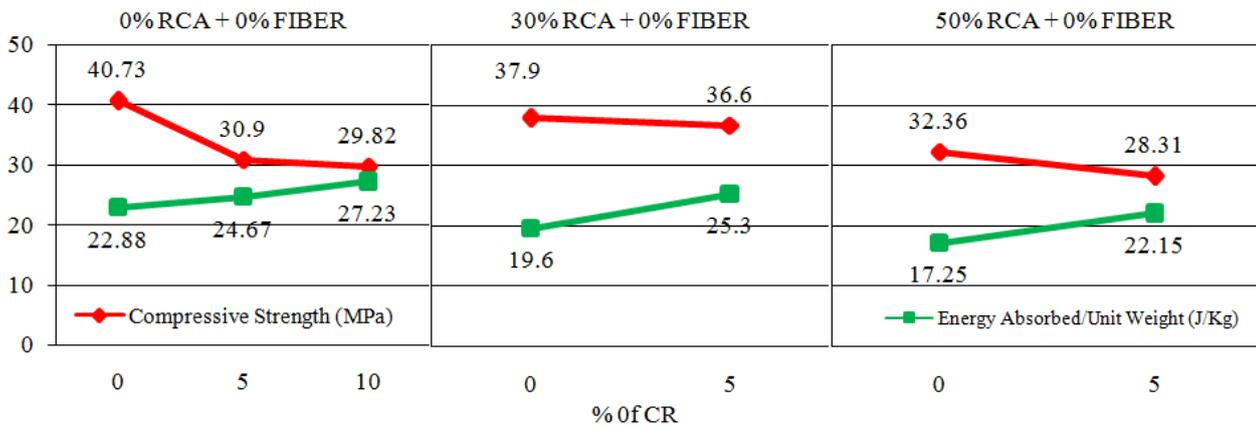
Figure 4. Effect of CR on compressive strength and energy absorption capacity.
