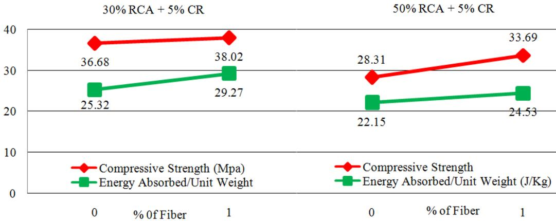
Figure 5. Effect of fiber on compressive strength and energy absorption capacity.
