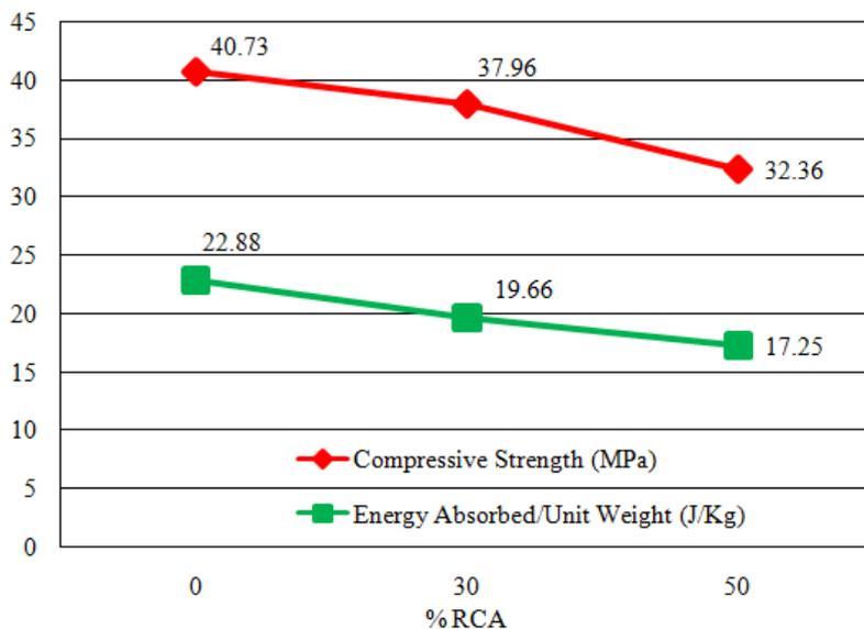
Figure 3. Effect of RCA on compressive strength and energy absorption capacity.
