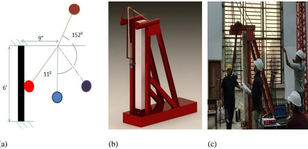
Figure 2. Customized Dynamic Impact Testing Setup (a) Working principle (b) 3D modeling (c) Original setup.
