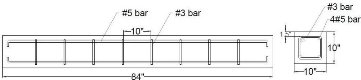
Figure 1. Reinforcement detailing of test specimens.
