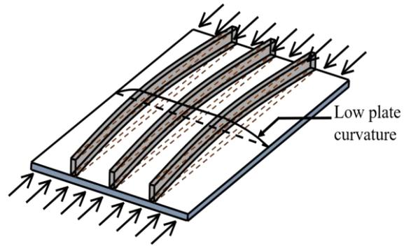
Figure 2. Stiffened plate with column-like behaviour in uniaxial compression.
