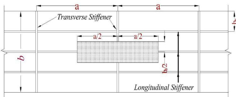
Figure 3. Stiffened plate model.
