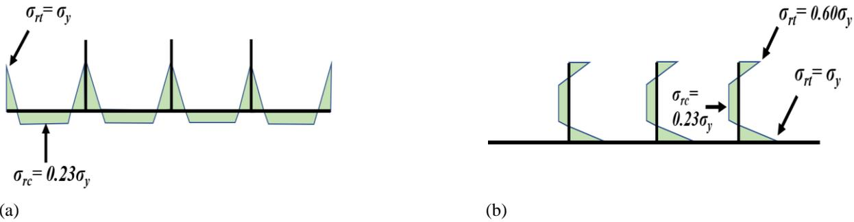
Figure 6. Residual stress distribution pattern for (a) bottom flange and (b) longitudinal stiffener.
