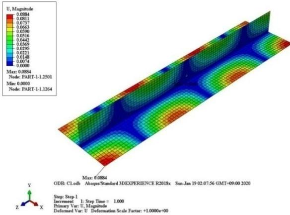
Figure 7. Simulation of two relevant modes to the stiffened plate model of  $R_R$  0.8 and  $\gamma_l/\gamma_{l.req} = 3$ .
