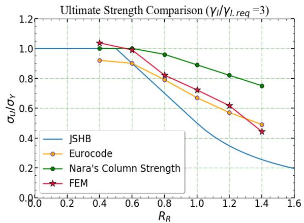
Figure 11. Comparison of ULS obtained by approximate solution with other design codes and proposal.
