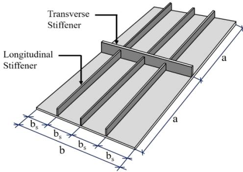
Figure 1. Wide stiffened steel plates.
