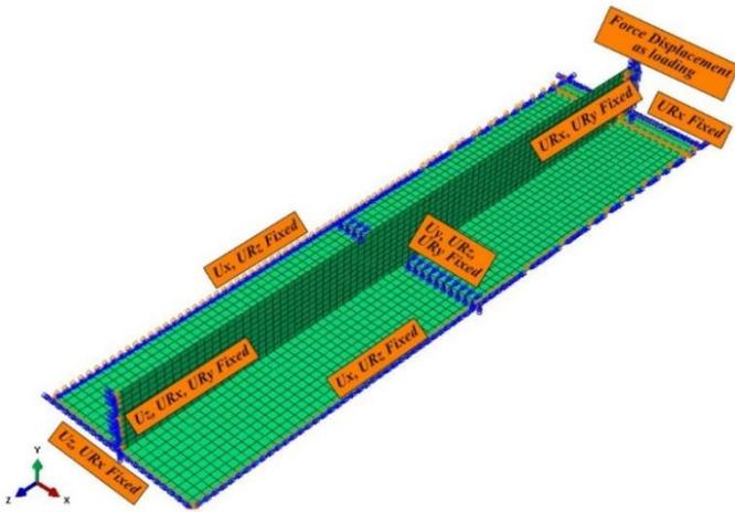
Figure 5. Boundary conditions of wide stiffened column model.
