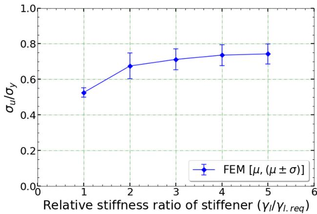
Figure 10. Variation of probabilistic strength with respect to relative stiffness ratio of stiffener at RR 1.2
