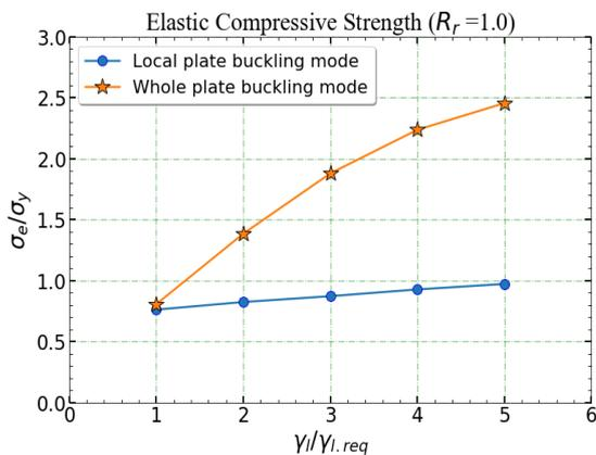
Figure 8. Effect of relative stiffness ratio of stiffener on elastic critical strength.
