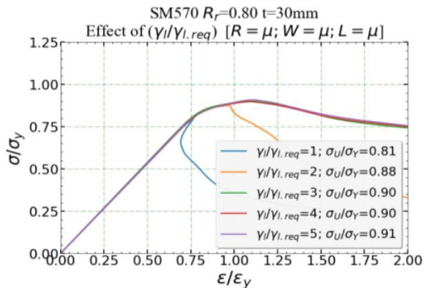
Figure 9. Effect of variation of relative stiffness ratio on ultimate buckling strength for  $R_R$  0.8
