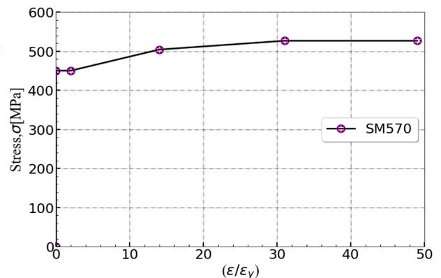
Figure 4. Idealized stress strain relationship for steel grade.
