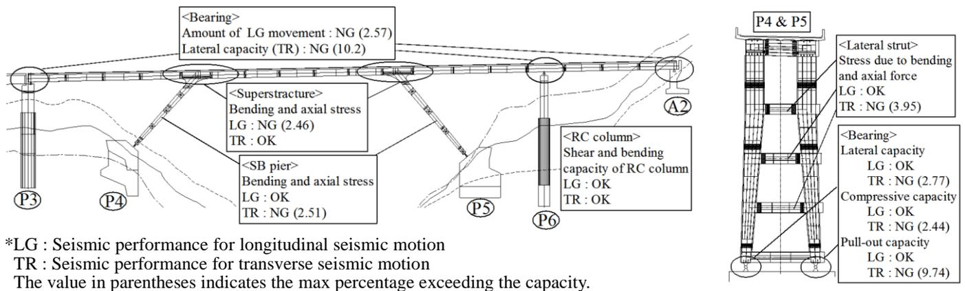
Figure 2. Outline of the seismic performance verification results (Up line).
