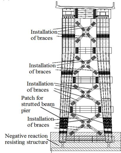
(2) Front view of the strutted beam pier.
