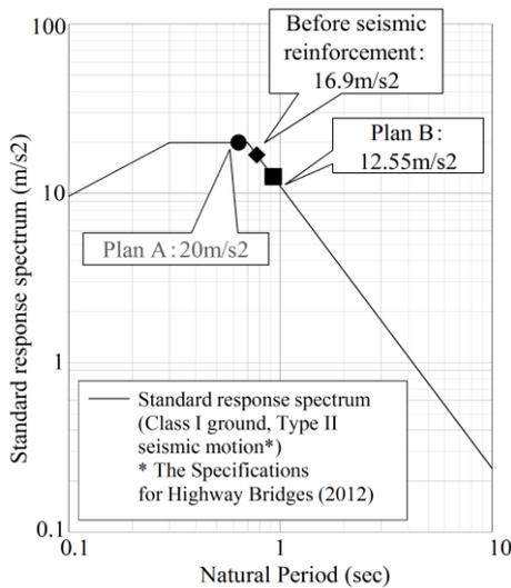
Figure 5. Standard response spectrum (Up line).
