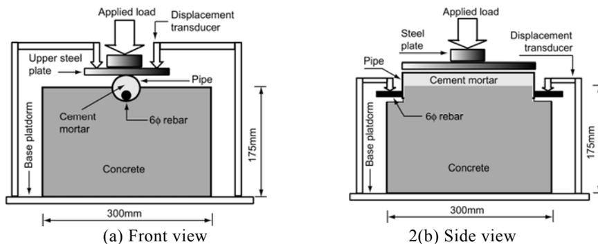
Fig. 2 Bearing test specimen
