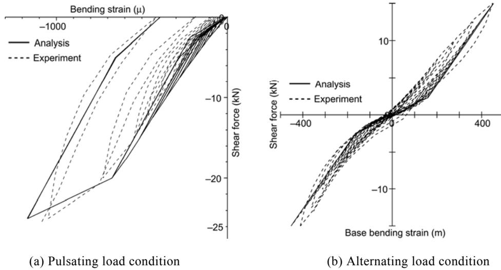
Fig. 8. Shear force-bending strain relations at base
