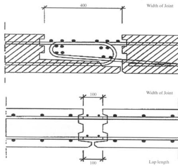
Exhibit – 3. Conventional joint (top) and the CRC filled joint (bottom) [3]
