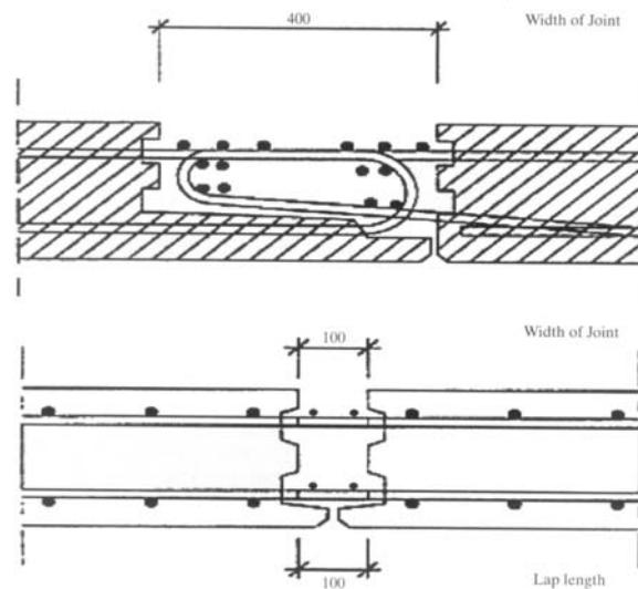
Exhibit – 3. Conventional joint (top) and the CRC filled joint (bottom) [3]
